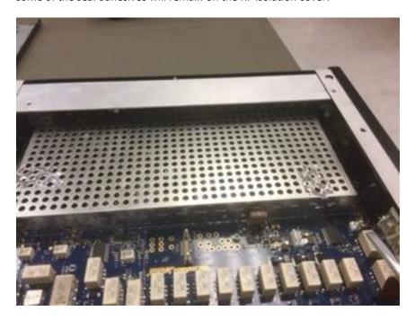
Take note of how the RF Isolation cover is seated in the shield housing's "teeth" (retaining tabs) for reassembly purposes.
