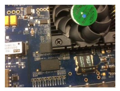
Carefully fold down the silver retaining clip so that it is flat against the MicroSD card. Slide the silver retaining clip towards the FPGA processor/fan assembly making sure that the MicroSD card does not slip or move in the socket. This will lock the MicroSD card in the card socket as shown below. This will result in the card not making proper contact with the card socket's electrical contacts causing the radio to fail to boot up.
