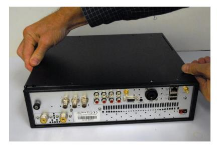
After reinstalling the bottom cover install the six (6) stainless steel (silver) **Bottom Cover screws** using the long portion of the #8 TORX wrench. The image below shows the installation of the Bottom Cover screws.
