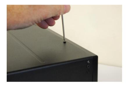
Using the long portion of the #8 TORX wrench install the three (3) short **Bottom Cover Side screws** on the **left** side of the FLEX-6000. Then install the remaining three (3) short Bottom Cover Side screws on the **right** side of the FLEX-6000. The image below shows the installation of the left side bottom Cover Side screws.
