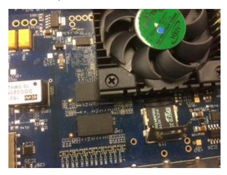
Using a non-metallic object to lift up on the end of the card nearest to the FPGA processor/fan assembly, the MicroSD card should easily lift out of the card socket so it can be removed.
