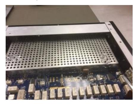
Once the RF Shield cover is installed, put two (2) new Warranty seal stickers on the RF Isolation shield in the same place where the previous stickers were located. **Be careful not to place any of the stickers on the PCB board.** The warranty seal sticker should only be on the silver RF Isolation housing and cover as shown below.
