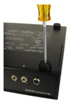
The finished re-installation of the bottom cover and chassis feet should look like the image shown below.
