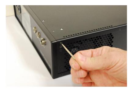
After removing the bottom cover side screws remove the six (6) stainless steel (silver) **Bottom Cover screws** using a #8 TORX wrench. Retain the bottom Cover screws for re-installation. The image below shows the removal of the Bottom Cover screws.
